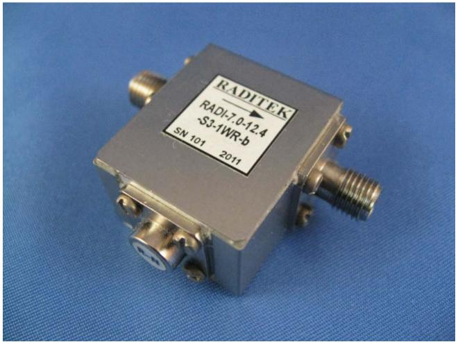
RADITEK'S Wideband Isolator Series: RADI-7.0-12.4-S3-1WR-b is a low cost key component to ensure high performance. Full band specifications include 20dB Isolation, 0.4dB Insertion Loss and VSWR 1.25:1 over the operating temperature -55 to +85 °C, Dimensions in mm: 21.3(W) x 24.7(L) x 15.2(H)
